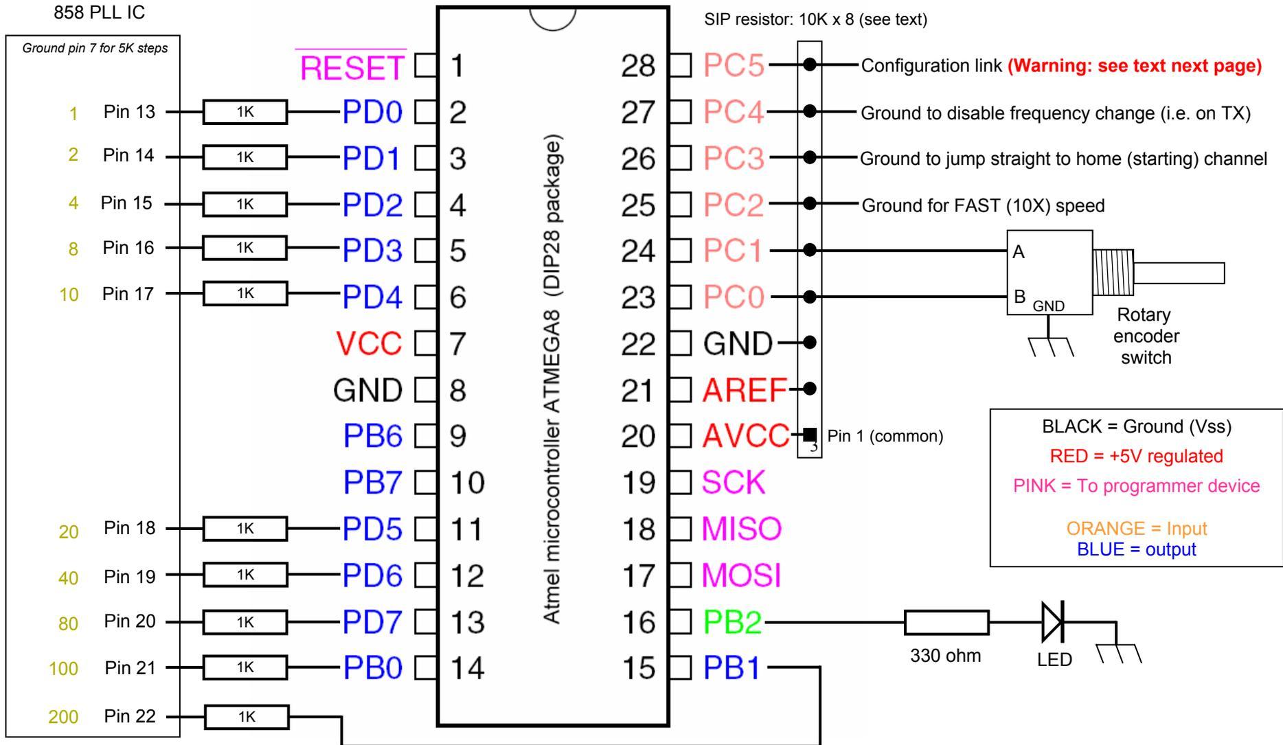
Bypass capacitors omitted from drawing for clarity. 100nF (0.1uF) MKT or ceramic capacitors from pins 7, 20, 21, 23, 24, 25, 26, 27, and 28 to ground are required. A 10uF electrolytic between VCC and ground. A 100uF electrolytic from the input of the 5V regulator to ground. These components **must** be fitted for correct operation!
